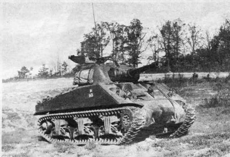
Short, fat assault gun on the Sherman tank is a 105-mm. howitzer. Long-barreled gun below is a high-velocity 76-mm. which calls for a bigger turret with roomier fighting compartment, larger hatches.
